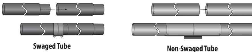
On the other hand, a non swaged tube design means that the clamp will act in part as the heat exchanger. The use of a large stainless steel clamp is often utilized to mask the fundamental problems that exist with this lesser securing method.
