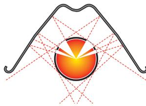
The shaded areas represent the sections of tube that emit infrared which reaches the space below. The sum of the angles of these sections is 315°. Dividing this number by 360° gives a percentage of the infrared which reaches the space below. This percentage is 87.5.
