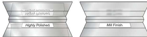
When radiant energy falls on a reflector's surface, it is either reflected or absorbed. Aluminum has a low absorption value and when combined with a polished surface, it will have a very high reflective value.
