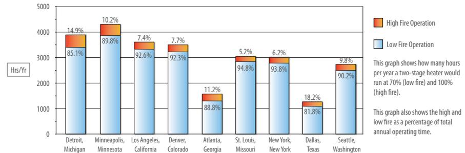
Unlike single stage heaters, two-stage operation allows for a 35% reduction in on/off cycles and has a documented 12% fuel savings over single stage heaters. Oftentimes, a 20% savings is realized. Two-stage heaters provide enhanced comfort levels and perform to the demands of the space. The two-stage operation also allows for faster heat recoveries, design flexibility and improved comfort levels.
